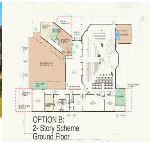
Schematic floorplan of the ground floor of Option B which contains the new gathering hall and some ground floor remodels:
